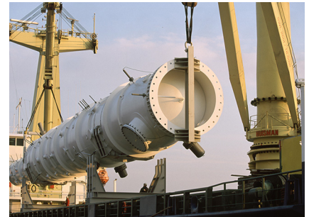
An Air Products LNG heat exchanger is loaded aboard a ship for transport to a global customer. A majority of the world's LNG is produced with Air Products' technology.
